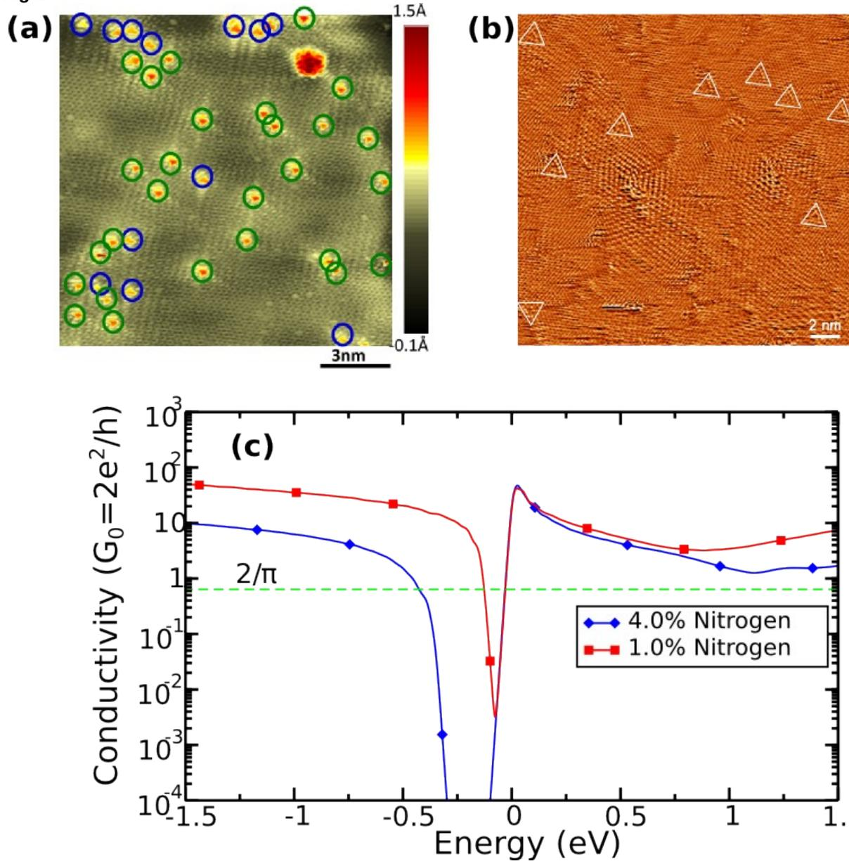
**Figure 1.** STM images of nitrogen doped graphene obtained by incorporation of N during growth: (a) single substitution [4], and (b) double substitution [5]. (c) Calculated semiclassical conductivities in graphene for various concentrations of N dopants randomly distributed in one sublattice [8].
